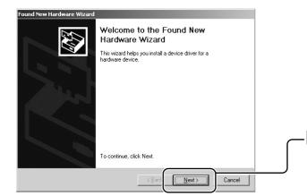
When a USB cable is connected, it is recognized as a new hardware, and a message is indicated.
