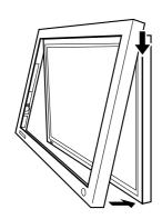
Never attach a plasma display onto the touch panel by placing the touch panel on a flat surface. Doing so may damage the infrared sensor on the touch panel
